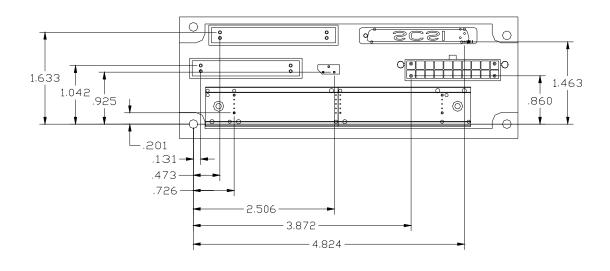
Figure 9-2: Peripheral Bay Board (Chassis Side) Connector Layoui
